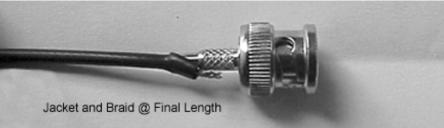
Finally, the outer ferrule is slid down the coax to compress the tag-end of the outer jacket and the braid between the two ferrule bodies. The outer ferule is then crimped firmly and the heat shrink tubing is put in place over the outer ferrule and the final 1/4 inch or so of the cable. I much prefer the heat shrink (available from Eur-Am) with heat-activated adhesive on the inner surface of the tubing. This product helps to provide mechanical reinforcement to the cable-connector joint.
