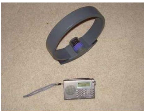
Facing Orientation - Eton e100 and Terk loop
