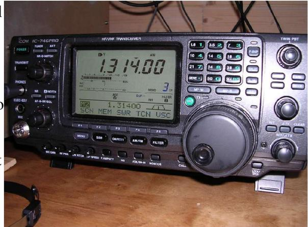
So then. My Icom IC-746Pro Receiver has a sensitivity of 0.6uV in the MW band (preamp 1 fixed on, preamp 2 not available on MW). My filter settings are 9.8/6.8/3.4 kHz on AM (nominally 9, 6 and 3 kHz), and 3.6/2.8/2.2 kHz on SSB. AGC release times on AM are 0.3/3.0/5.0 seconds (factory default being 3/5/7 seconds). I am a MW DX-
