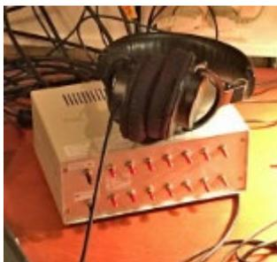
*A switchbox with amplifiers and fitted for 14 antennas, made by Stefan Wikander.*
